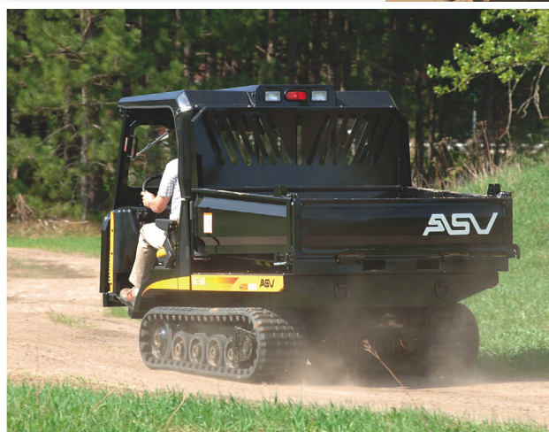
With its suspended undercarriage, the Scout provides a supple ride at top speed.
