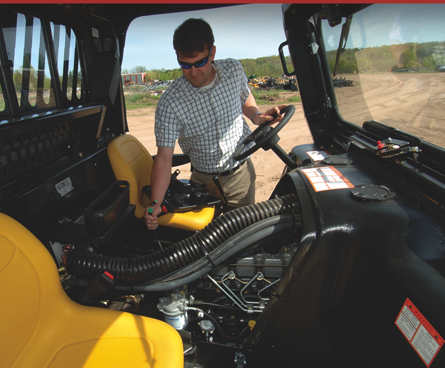
Design details, clockwise from upper left: With the Scout's engine cover removed, ASV's Lemke holds the two simple wiring harnesses that connect the auxiliary-hydraulic joystick to its control valve; a side compartment gives access to routine-maintenance points and to the fuel filler for the Scout's 30-gallon tank; and a heavy-duty cover for the front auxiliary-hydraulic panel includes a bail for towing or tie-down.
