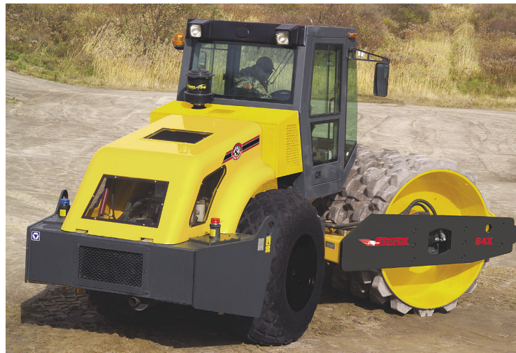
Above: The steeply sloped, contoured, fiberglass hood of the Rhino 84X enhances visibility rearward and provides easy access to service points.
