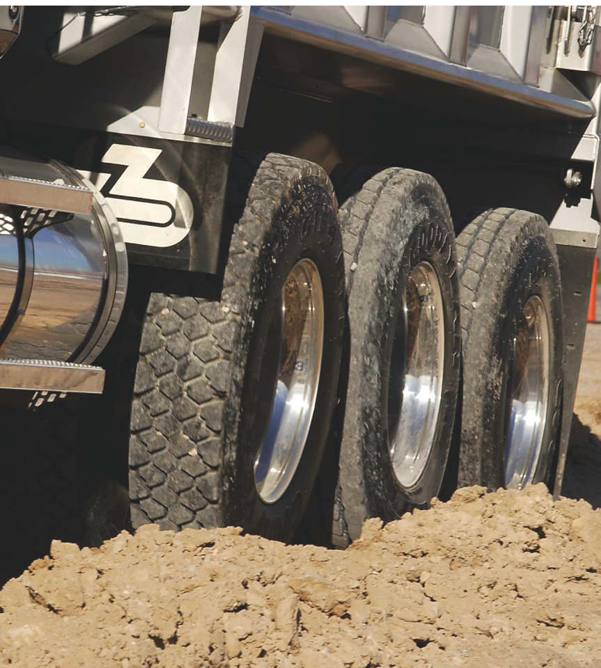
Selecting the right tread pattern for tires used on the often-hostile road surface of a construction site, as shown here on this dump truck, can help resist “chipping and chunking” caused by stones and gravel. (Photo: Goodyear Tire & Rubber.)
