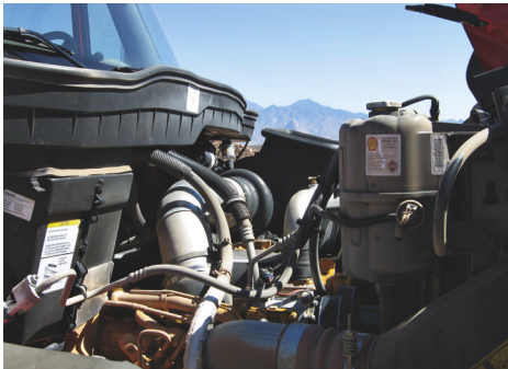
Cat C13 engine lurks behind splash guards and under the air cleaner, but most everyday check items are accessible.
