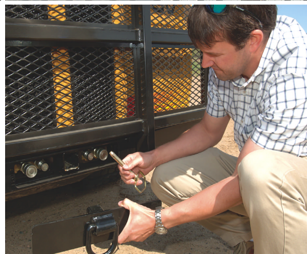
Design details, clockwise from upper left: With the Scout's engine cover removed, ASV's Lemke holds the two simple wiring harnesses that connect the auxiliary-hydraulic joystick to its control valve; a side compartment gives access to routine-maintenance points and to the fuel filler for the Scout's 30-gallon tank; and a heavy-duty cover for the front auxiliary-hydraulic panel includes a bail for towing or tie-down.
